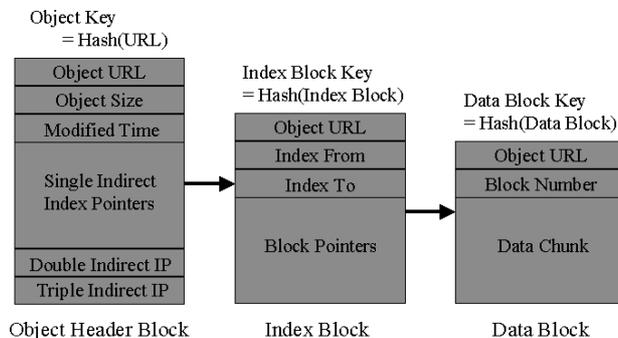
Fig. 2 The structure of a large sized object.
